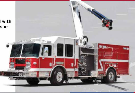
The Talon offers many options to maximize fire scene capabilities, such as color and thermal image camera systems, elevated lighting and piercing nozzle.
